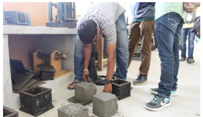
Concrete cube Casting
